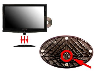
2. To remove the stand remove the screws in the circled area and the neck will come off.
